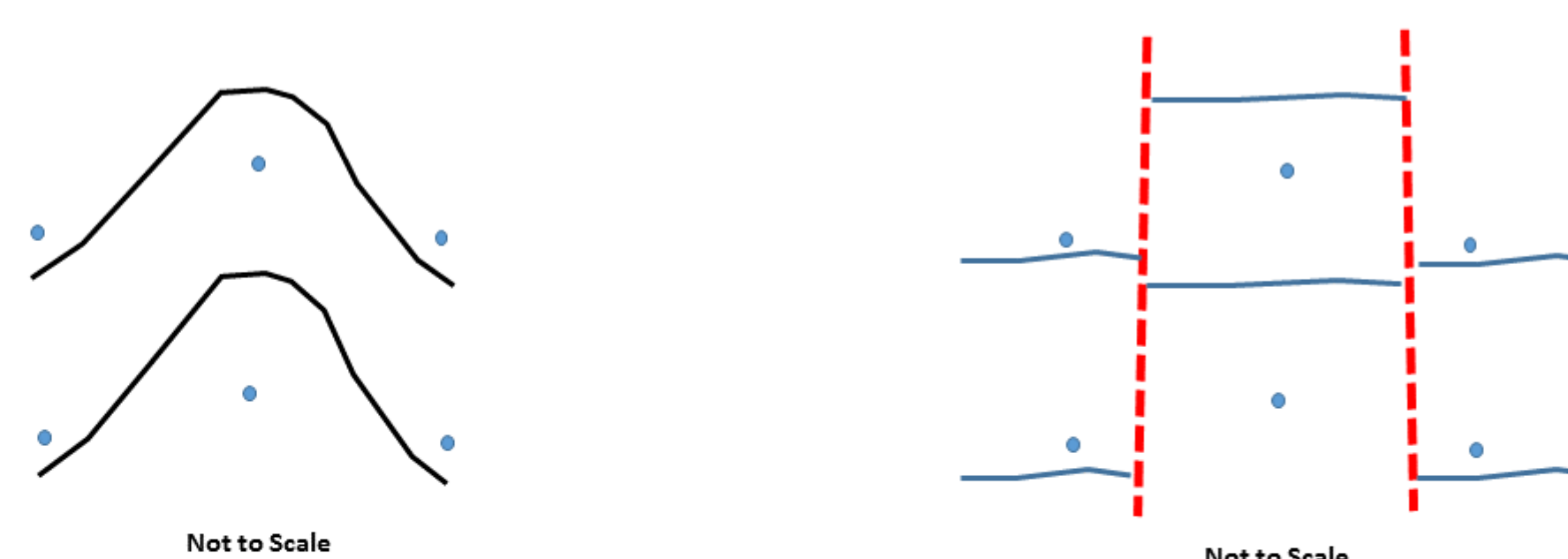
Figure 5 & 6_ When we were studying hydrogeology, we were told that if the water level contours looked like the one on the left; then we need to check the geology it may actually be like the one on the right.
